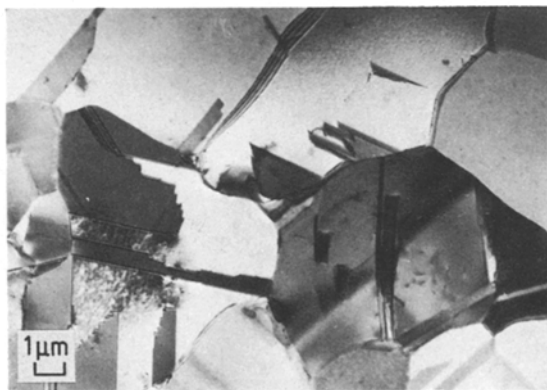
Figure 4 The microstructure of a specimen annealed at 350^\circ\text{C} for 50 sec after cold rolling (TEM).
